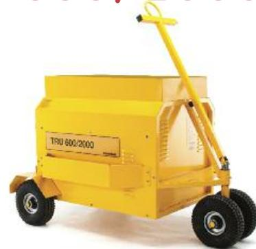
The Powervamp TRU600/2000 is an advanced transformer rectifier unit delivering 28.5V at 600A continuous and 2000A peak for engine starting. Regulation is achieved using additional thyristor control BEFORE the transformer, to achieve a clean output with less ripple than traditional TRUs. The TRU600/2000 is capable of worldwide operation as standard from the factory.
